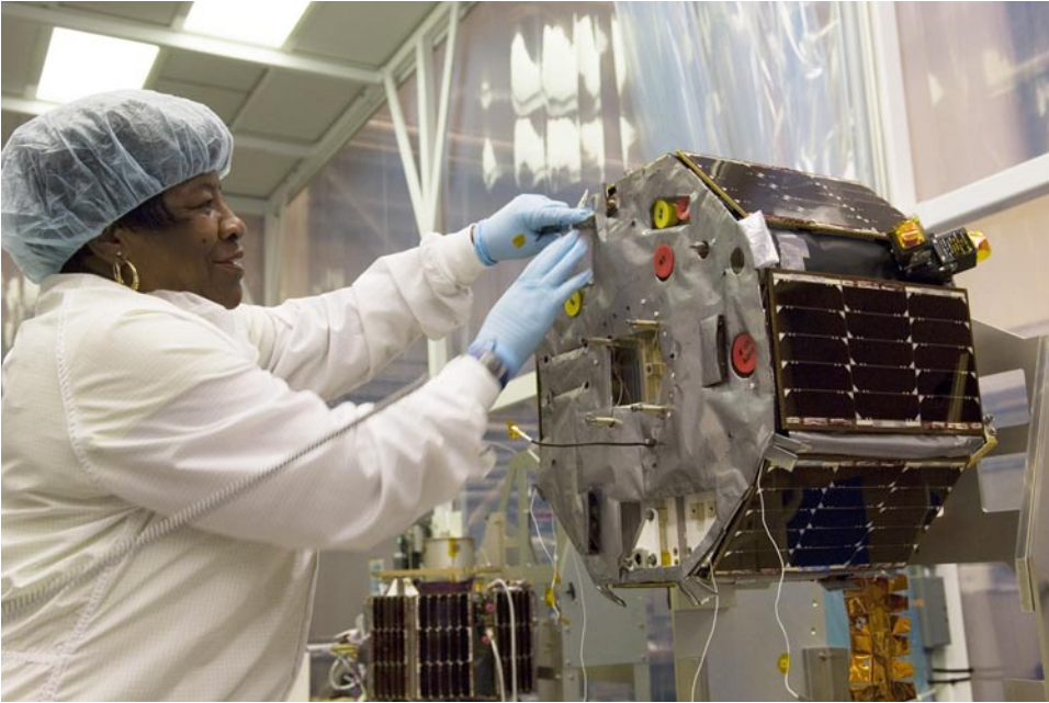
Caption: Helen Johnson, a spacecraft technician at NASA's Goddard Space Flight Center, works on one of the three tiny Space Technology 5 spacecraft in preparation for its technology validation mission.
