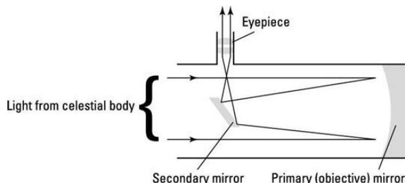
**Reflecting Telescope Design.**
