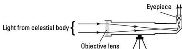
**Refracting Telescope Design.**
